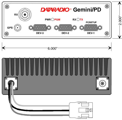
Figure 5 - Front and rear panels
